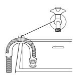
The end of the drain hose must always be **ventilated**, i.e. the inside diameter of the drain pipe must be larger than the outside diameter of the drain hose.
